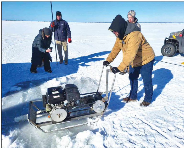
This sled saw is powered by a 13-hp motor and cuts with a 42" chainsaw bar.
