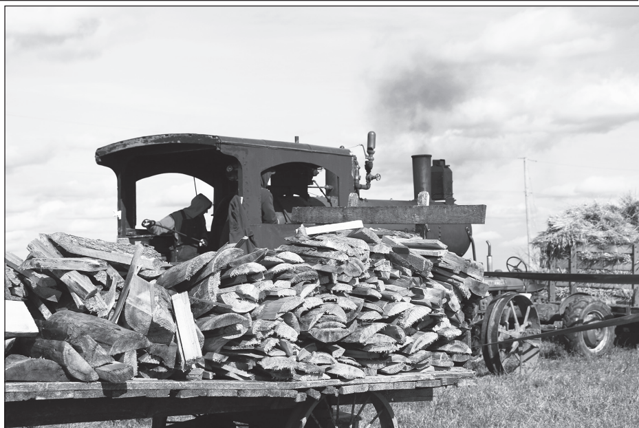
Wood is burned to create steam to power a threshing machine.
