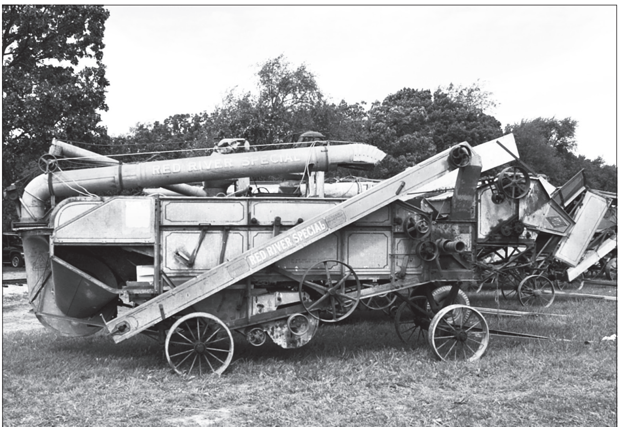
The Oliver Red River Special, made in the late 1920s, early 1930s. The machine was capable of threshing 1,500 bushels a day.
