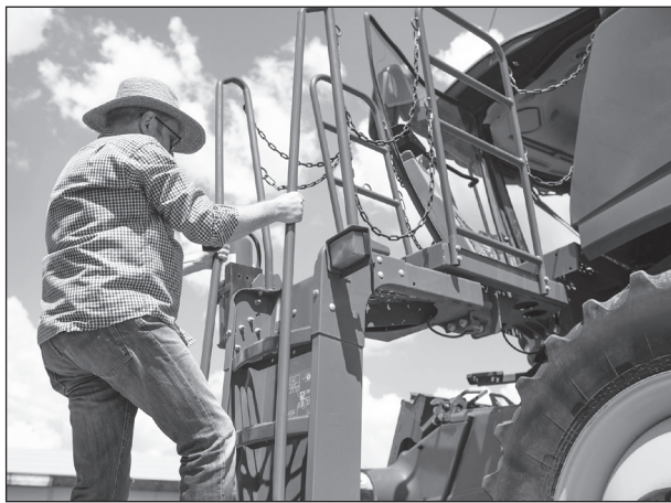
Use the three-point system to prevent slips and falls from ladders. MASTER1305
