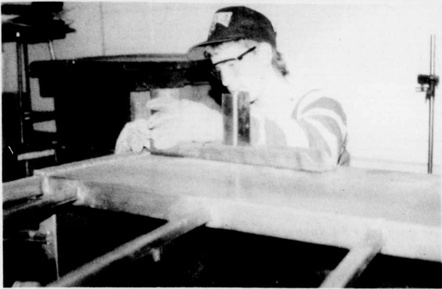
Using his welding skills, Doug Neumann is constructing a 16' cow feeder. Planning, cutting, forming, and assembly are all part of his job.
