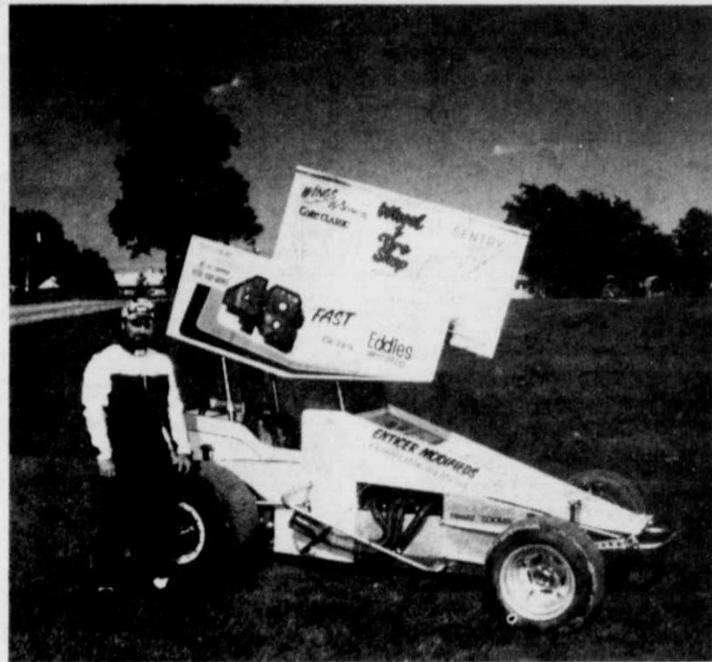
Erv Waala III enjoys the "Enticer," complete with 406 Chevy engine and '57 Chevy body.
