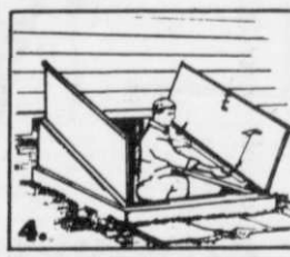
Secure to concrete and caulk.
