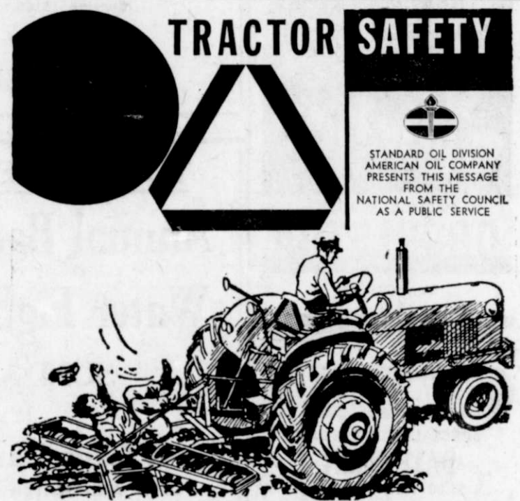
Don't allow riders on tractor, drawbar, or towed equipment unless a seat is provided for them. Reprint From Booklet — Tractor Safety.
