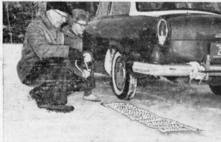
1. W. B. (Walt) Lashar, Jr., chairman of National Safety Council test committee, shows Marion Olund, Clintonville, Wis., the first step. Spread chains on the ground to remove tangles. Reinforced chains are best, and the projecting teeth or cleats should be up.
