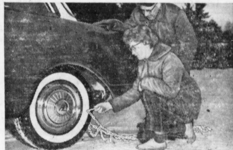
2. Then put end links of side chains on loops of "applicator" and push onto tire as shown. No jack is needed.
