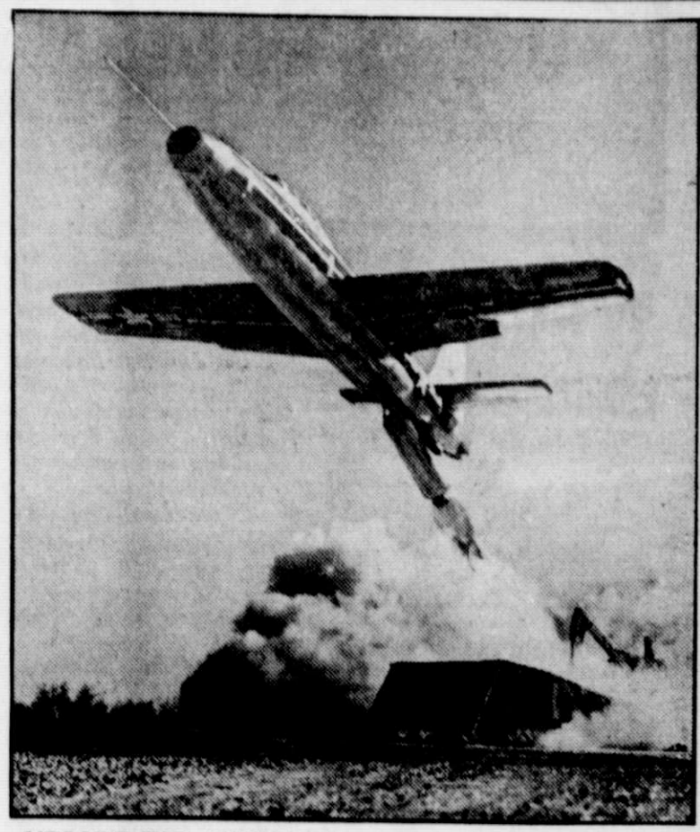
AIRPORT FOR ANYWHERE —F-84 Thunderjet is first plane to be hurled into a new era of military aviation from bed of a specially designed truck near Baltimore, Md. With assist from a booster-jet bottle seen hanging beneath tail, plane, with engine at full throttle, is boosted to the 120-m.p.h.-plus take-off speed in a few feet, rather than the eight-thousand-foot-plus runway usually needed. Highly mobile technique was developed through joint efforts of the U. S. Air Force and Glenn L. Martin Company and may someday make long fighter airstrips obsolete.
