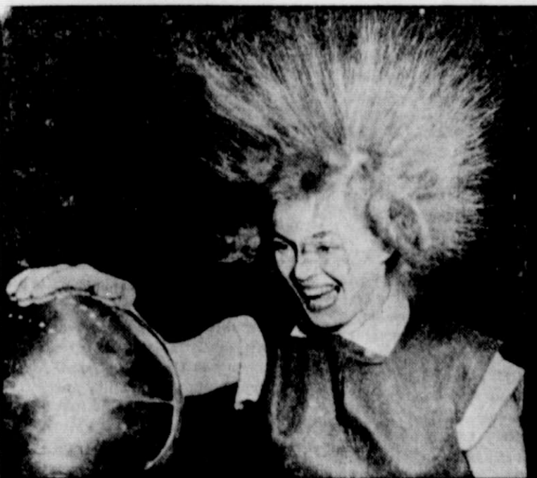
CAN'T DO A THING WITH IT —Thelma Chaney is going to have trouble with her hairdo just as long as she has her hand on this Van de Graf electrostatic generator, at the University of Washington, in Seattle. Static electricity with which she's charged drains into atmosphere through her hair.
