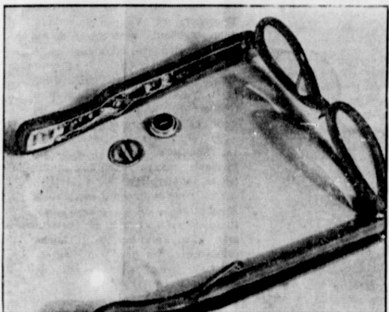
LOOK TO LISTEN —Powered by a tiny battery to right of dime, shown for comparison, a new-type hearing aid which masquerades as an eyeglass frame is now in production. Clear plastic tube, shown on lower ear frame, conducts amplified sound to the wearer's ear. The battery, which screws into ear frame, has a life-in-use of about 180 hours. Frames may be fitted with clear glass for those with good eyesight who yet want to dispense with paraphernalia of more conventional hearing devices, according to the Dobbs Ferry, N. Y., manufacturer.
