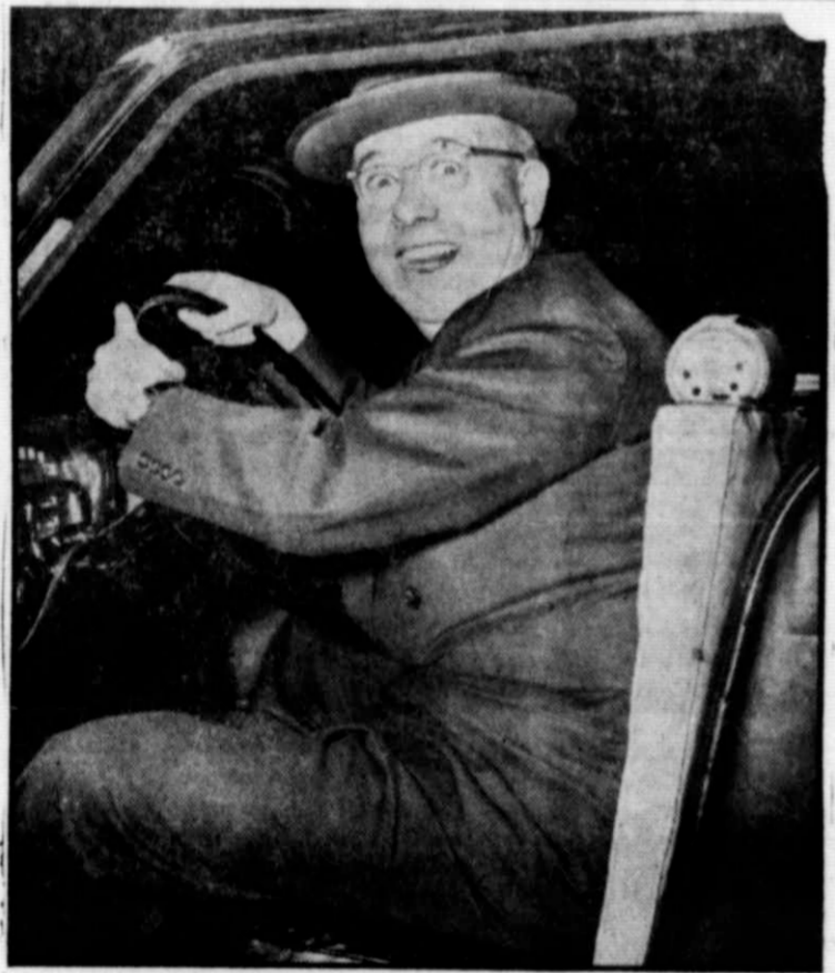
SHAKE THAT AWAKES—Drowsy drivers could disappear from the nation's highways when and if the "carriage" becomes widely used. The device, shown above being tested by New York news-writer Ed Wallace, is powered by a small electric motor attached to the cigaret-lighter outlet on the dashboard. The porous plastic material massages the motorist's back when the current is on, keeping him awake.
