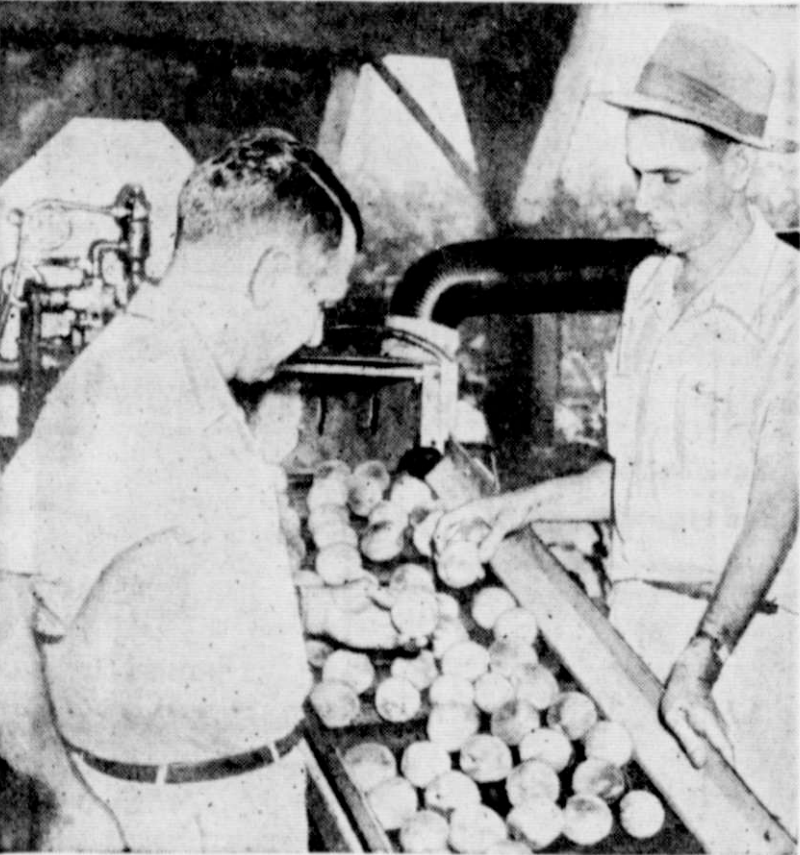
CLEAN-SHAVEN PEACHES . . . Soon, thanks to this machine being tried in Spartansburg, S. C., your peaches will come to you in shining nudity. The gadget is a peach polisher designed to take the fuzz off the peach and apply a thin coat of wax to seal in the natural flavor of the fruit and reduce shrinkage. Revolving brushes do the job. Examining some newly-shaved peaches as they come through the machine are Les Collier and Ben Gramling. No, an electric razor won't work.
