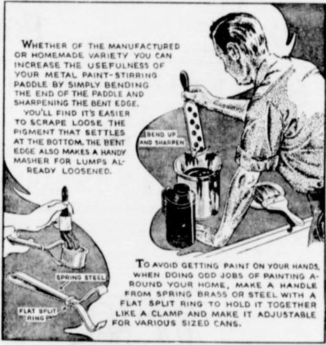
WHETHER OF THE MANUFACTURED OR HOMEMADE VARIETY YOU CAN INCREASE THE USEFULNESS OF YOUR METAL PAINT-STIRRING PADDLE BY SIMPLY BENDING THE END OF THE PADDLE AND SHARPENING THE BENT EDGE. YOU'LL FIND IT'S EASIER TO SCRAPE LOOSE THE PIGMENT THAT SETTLES AT THE BOTTOM. THE BENT EDGE ALSO MAKES A HANDY MASHER FOR LUMPS ALREADY LOOSE.
