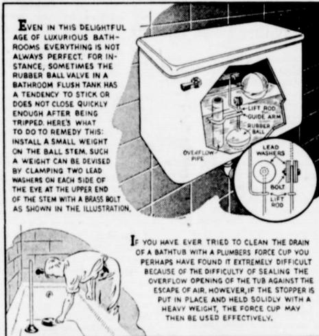
EVEN IN THIS DELIGHTFUL AGE OF LUXURIOUS BATHROOMS EVERYTHING IS NOT ALWAYS PERFECT. FOR INSTANCE, SOMETIMES THE RUBBER BALL VALVE IN A BATHROOM FLUSH TANK HAS A TENDENCY TO STICK OR DOES NOT CLOSE QUICKLY ENOUGH AFTER BEING TRIPPED. HERE'S WHAT TO DO TO REMEDY THIS: INSTALL A SMALL WEIGHT ON THE BALL STEM. SUCH A WEIGHT CAN BE DEvised BY CLAMPING TWO LEAD WASHERS ON EACH SIDE OF THE STEM WITH A BRASS BOLT AS SHOWN IN THE ILLUSTRATION.
