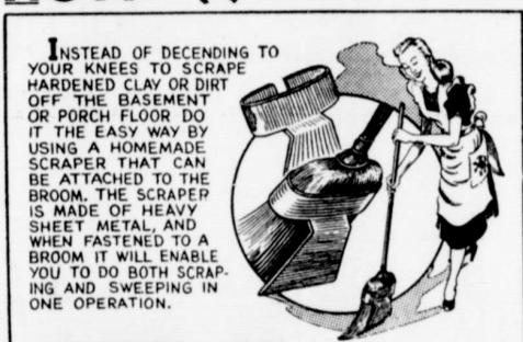
INSTEAD OF DECENDING TO YOUR KNEES TO SCRAPE HARDENED CLAY OR DIRT OFF THE BASEMENT OR PORCH FLOOR DO IT THE EASY WAY BY USING A HOMEMADE SCRAPER THAT CAN BE ATTACHED TO THE BROOM. THE SCRAPER IS MADE OF HEAVY SHEET METAL, AND WHEN FASTENED TO A BROOM IT WILL ENABLE YOU TO DO BOTH SCRAPING AND SWEEPING IN ONE OPERATION.
