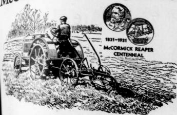
McCormick-Deering 10-20 Tractor prondes power in abundance for general farm It pulls two plows under all reasonable mins and travels at good speed while plow-for its size, the 10-20 has a great capacihork—you can apply its power three ways dawbar, belt, or power take-off-to operate mety of equipment throughout the year. he surprising strength of the 10-20 is due
