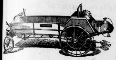
THE new McCormick-Deering No. 4-A all-steel spreader is convenient, low to the ground, simple, and compact. features a galvanized, rust-resisting, copperized, nonwarping, heavy-gauge steel box of 60 to 70-bushel capacity. Fight roller bearings and Zerk lubrication, combined with effect alignment of all parts, make this new all-steel preader unusually light in draft. Two horses can haul apacity loads in it all day long.
