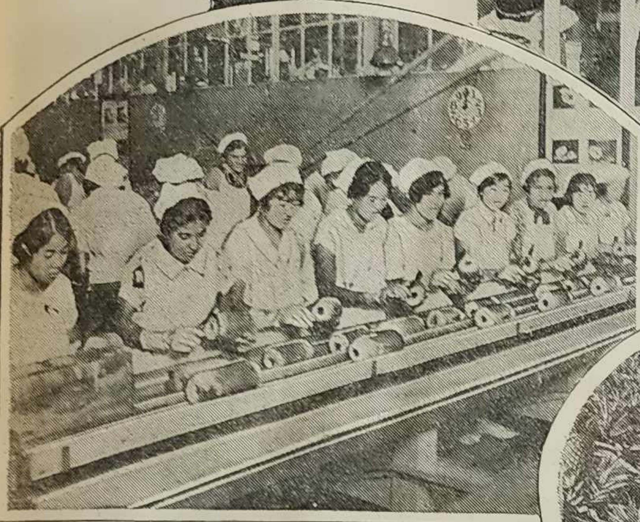
Girls wearing white caps and rubber gloves trim the pineapple as it comes from the ginaca machine.
