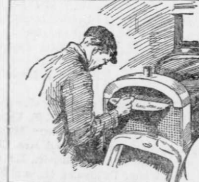
Incision in Radiator, After the Shell Is Removed, Gives Access to Obstructing Particles.
