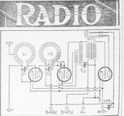
Three-Tube Receiver Unexcelled for Distance, Volume and Tone, Square Wound Toroidal Coils Give the Circuit Selectivity.
