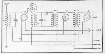
The Electrical Schematic Diagram of Toroid RF Simple Three-Tube Set, Using Crystal Detector.
