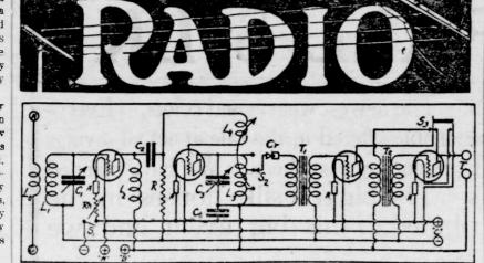
The Wiring Diagram of an Impedance-Coupled Radio Receiver of Unique Design-Carborundum Crystal Detector Insures Stable Operation.
